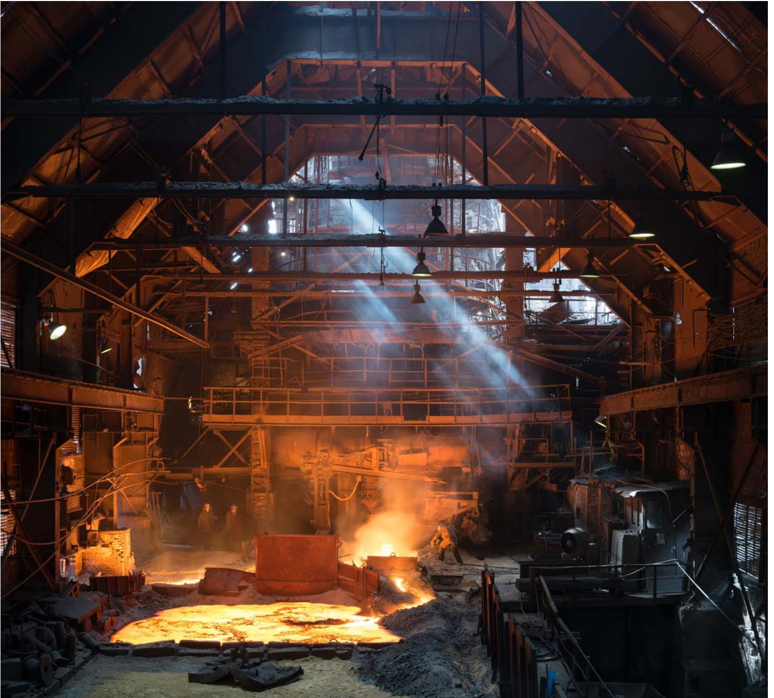
Kosaya Gora ironworks, south of Moscow: Casting house during the tapping of a small capacity blast furnace made for ferromanganese production. Casting into a sand pit is an ancient process of iron making which doesn't now exist anywhere in Europe. The intense heat was unbearable. Photo: Viktor Macha
